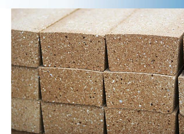
The dimensional tolerances of bricks generally conform with the PRE/R23 Recommendation ("Dimensional tolerances of dense and insulating refractory products").
